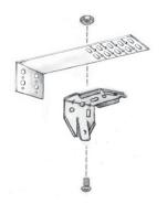
If you need to project the shade out from the mounting surface, use the supplied nuts and bolts to attach mounting brackets to the desired position in the extension bracket. With pliers, bend and break the unused part of the extension bracket. Attach extension brackets to mounting surface, making sure brackets are spaced as noted above.
