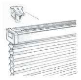
Larger shades may require additional brackets. Space additional brackets equally and align with the end brackets. Note placement of components inside headrail. Brackets must be placed in the open areas between components to avoid interfering with the operating mechanism. Mark these locations on top of window frame for inside mount or on wall for outside mount.
